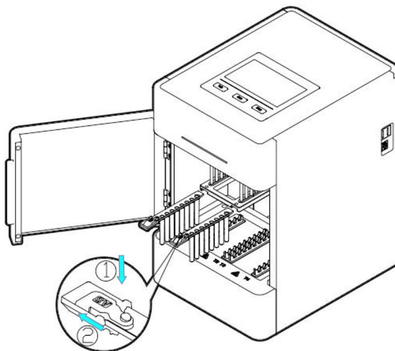
Fig 12 Remove magnetic rod's tip
