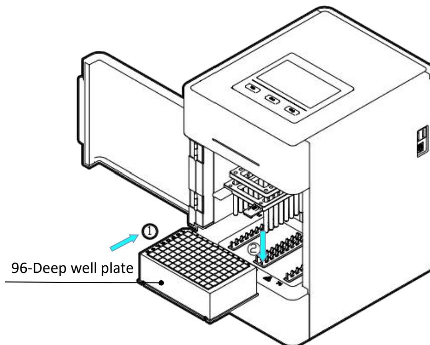
Fig 9 96-Deepwell plate installation
