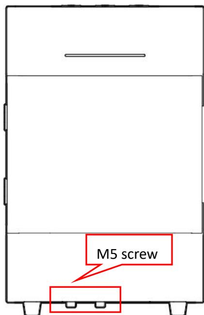
Fig 8 Remove fixing screw
